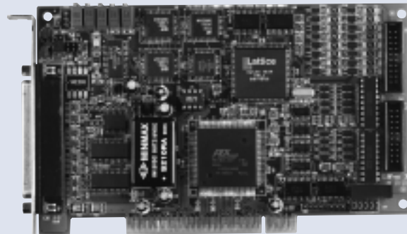
PCI-9114DG: 32-CH, 16-bit Normal Gain DAS Card
